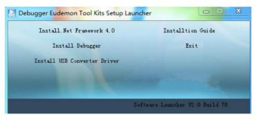
For the initial use of this debugger eudemon, it is required to install .Net Framework 4.0, USB Converter Driver, and Debugger.
