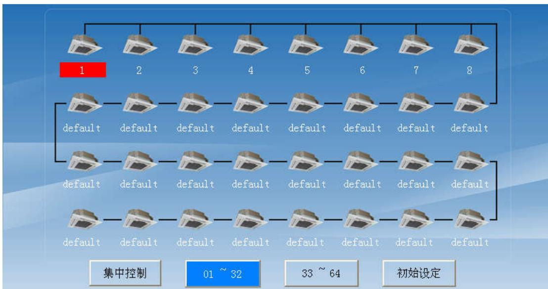
Above picture is "01~32" control interface, and this interface can show startup&working status from address 1 to 32 of super uno AC. If super uno AC named "default", this super
