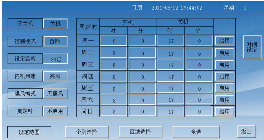
Above picture is "centralized control setting" interface, and after user finish setting up parameter, it can choose "single choose" operation, "zone choose" operation, and "all choose" operation for super uno AC.
