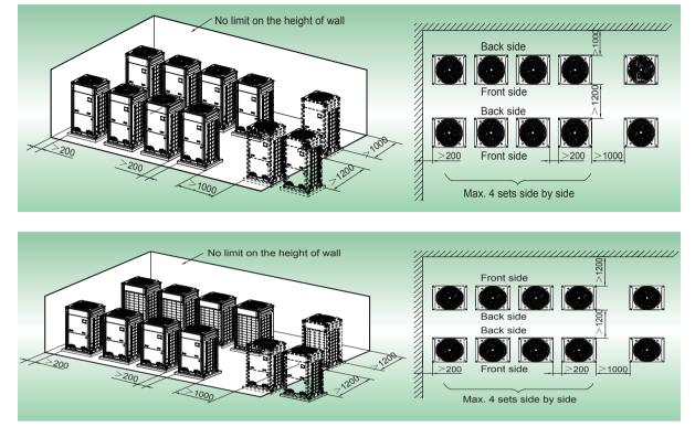
be installed towards the same direction or reverse direction.
