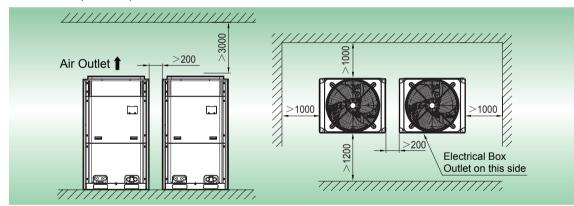
Installation space requirements for triple-module unit
