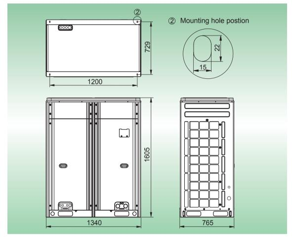
External and installation dimensions of SMZU135V2AI and SMZU150V2AI:
