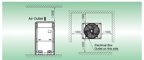
Installation space requirements for the dual-module unit
