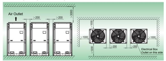
Installation space requirements for quad-module unit
