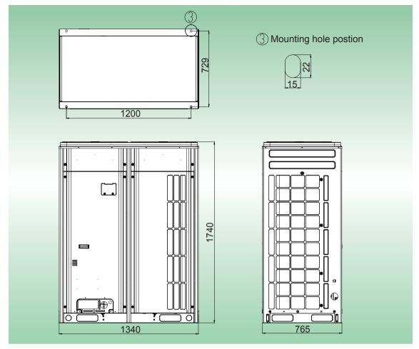
External and installation dimensions of SMZU175V2AI, SMZU190V2AI and SMZU215V2AI:
