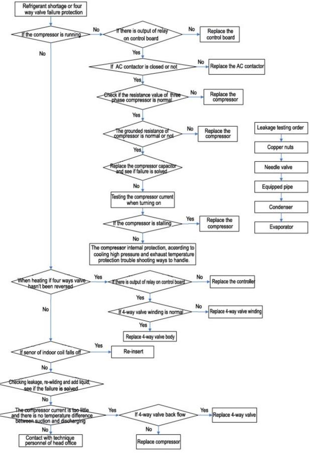
Refrigerant shortage or four way valve failure protection
