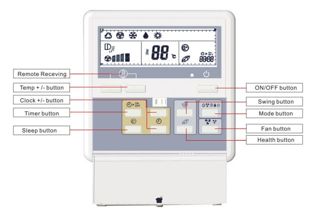
ON/OFF button: Switch the unit ON/OFF.
