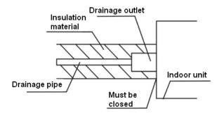
Heat insulation material: rubber insulation pipe with the thickness of more than 8mm
