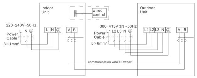
Note: Indoor machine power can also be introduced from the bonnet, which will indoor the L received the outdoor L1, L2, L3 either one,
