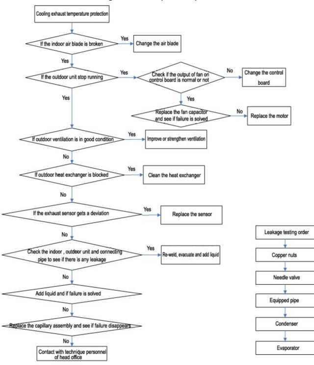
**Cooling exhaust temperature protection**
