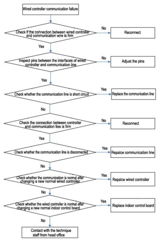
Wired controller communication failure
